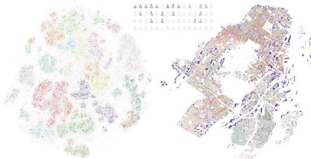
Figure 1. Clusters of Building Form in Montreal Using Deep Learning Model in Data Space (left) and Map Space (right)
